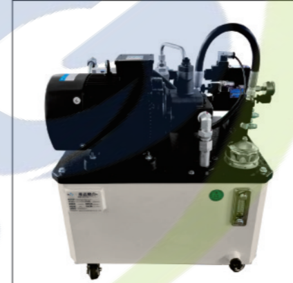
机床液压系统 Machine tool hydraulic system
